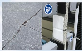
No leakage of the film in case of crack of the substrate to function as waterproofing. It is ensured by the cohesion of the polymer.
