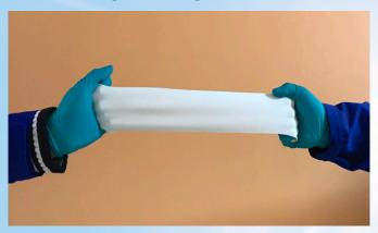
The balance of tensile strength and elongation is a very important parameter to get a high performance roof coating, as it relates to toughness and elasticity of the cured membrane.
